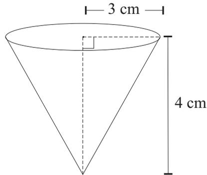
The diagram above shows a vessel in the shape of a cone of radius 3 cm and height 4 cm. Water is poured into it at the rate of  $10 \text{ cm}^3/\text{s}$ . Find the rate at which the water level is rising when the depth is 2 cm.
